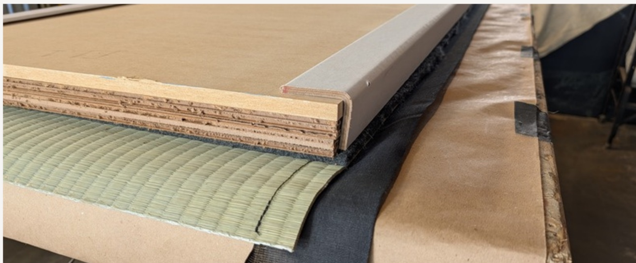
TOP: FELT LAYER TO CUSHION GOZA, BOTTOM: LAYERS WITH GOZA IN PLACE - LAID UPSIDE DOWN
